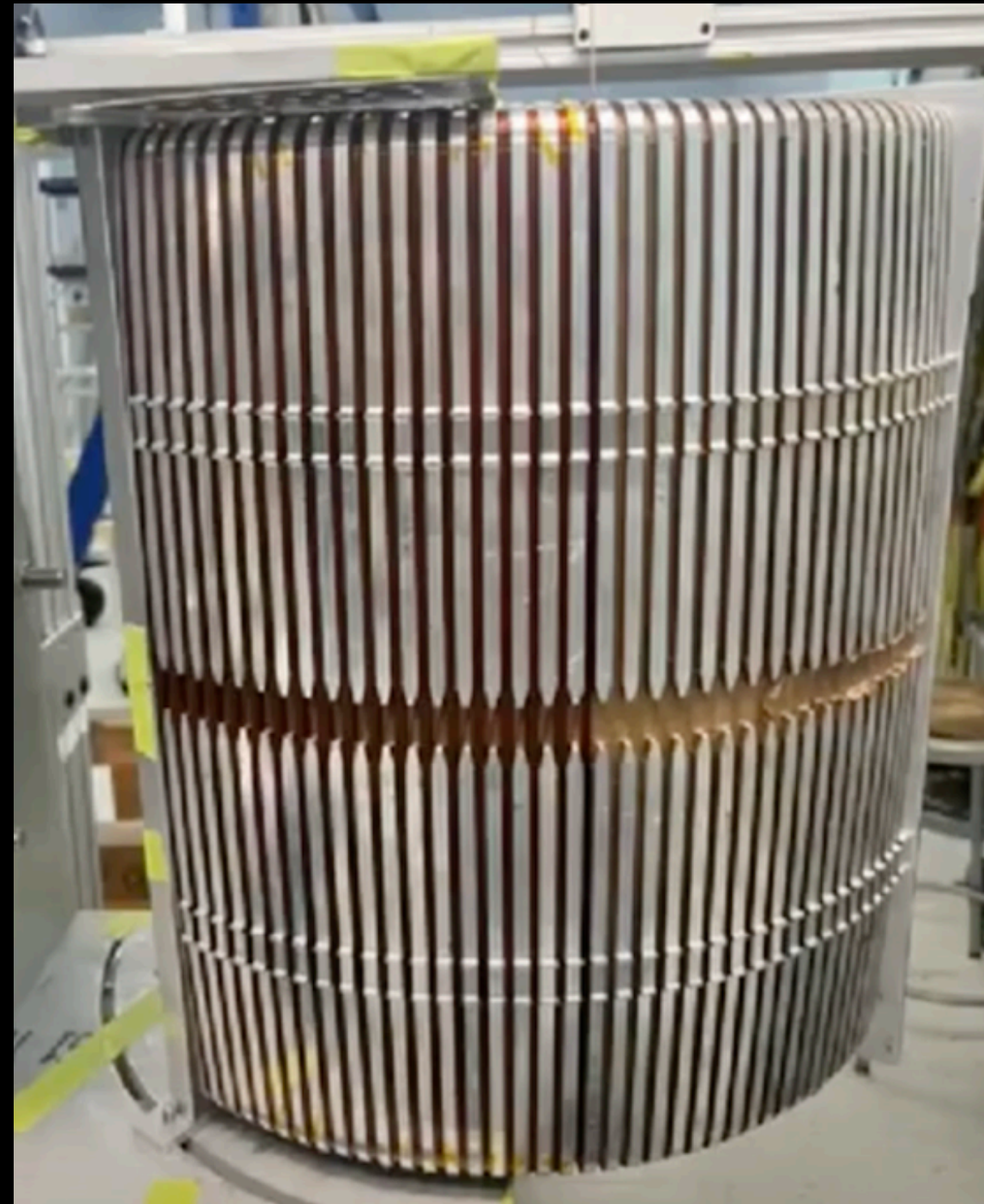
Mandrel construction and winding Superconducting Systems Inc
