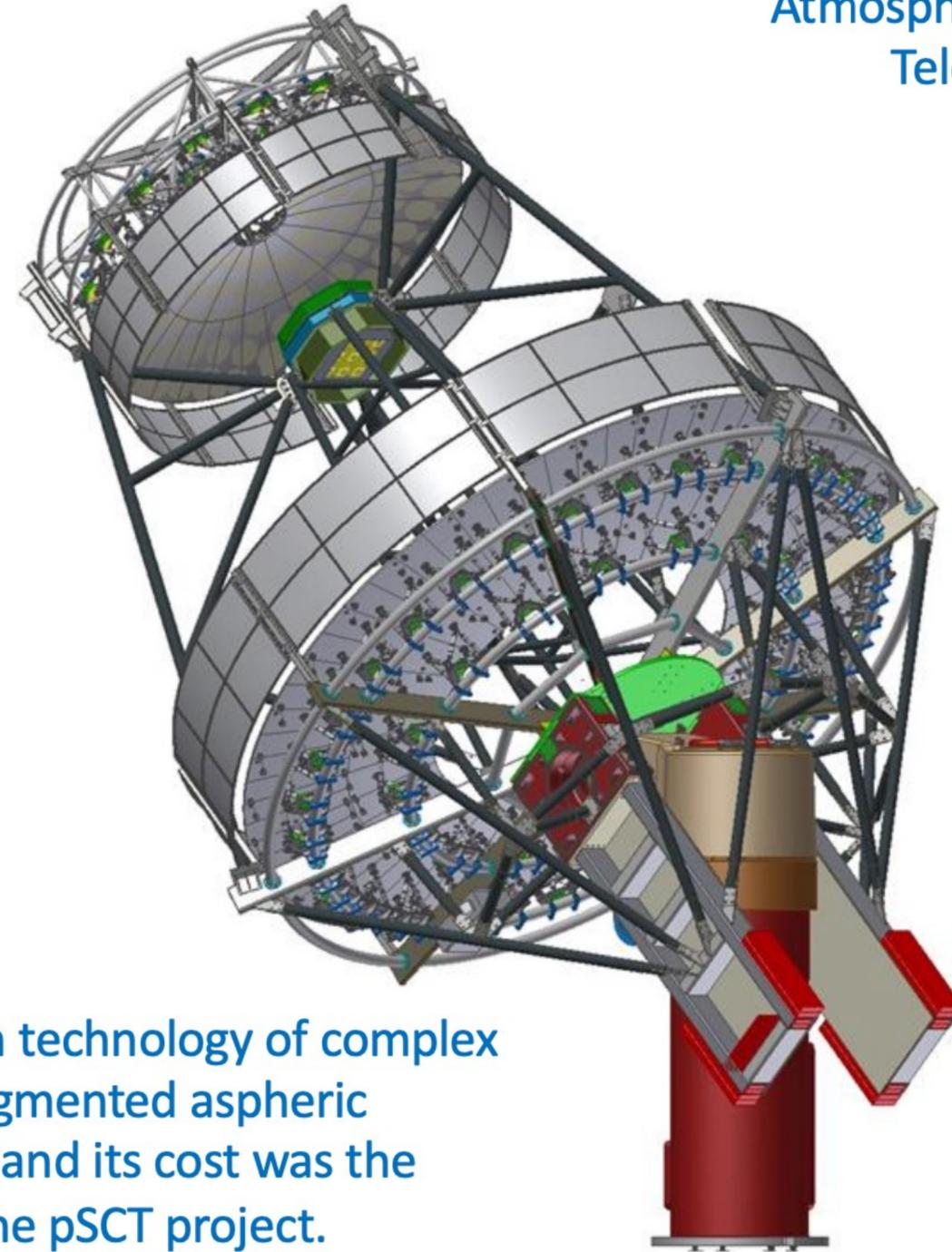
The fabrication technology of complex dual-mirror segmented aspheric optical system and its cost was the major risk of the pSCT project.
