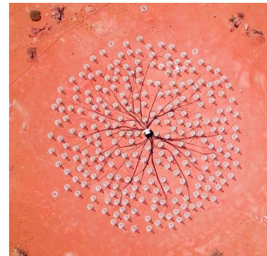
Prototype @MRO (256 antennas)
