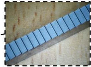
16x Curved Diffraction Gratings ( R \sim 170 )
