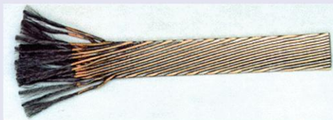
Rutherford cables: cross-section
