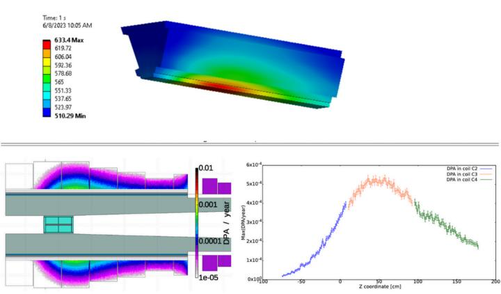
Fig. 6.5.1: 2D map of the displacement per atom (DPA) in the superconducting magnets of the target area (left) and the peak DPA in the coils most exposed to radiation (right).
