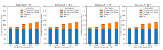
Cryogenic loads at different temperatures
