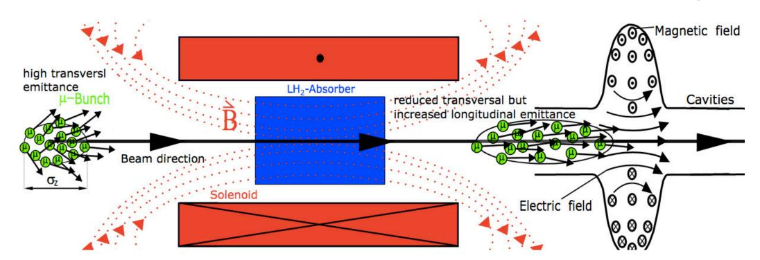
High field solenoids minimise betafunction and impact of multiple scattering
