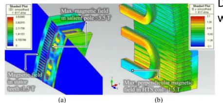
Design of 10 MW HTS wind generator
