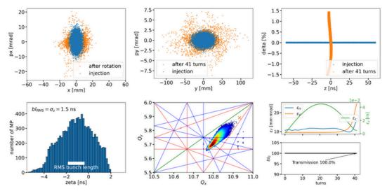
**Fig. 5.1.8:** Simulation of the full compression for one bunch at 5 GeV. Since this requires a 2 bunch solution scheme, this bunch has half of the full intensity shown in Table 5.1.1. Notice that at the end of the compression there is still some emittance blow up that need still to be addressed.
