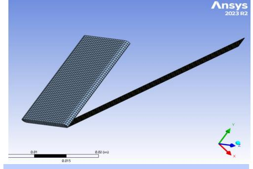
Segment of flat rounded-edge cable with tape contact, pre-winding simulation, after FE meshing.
