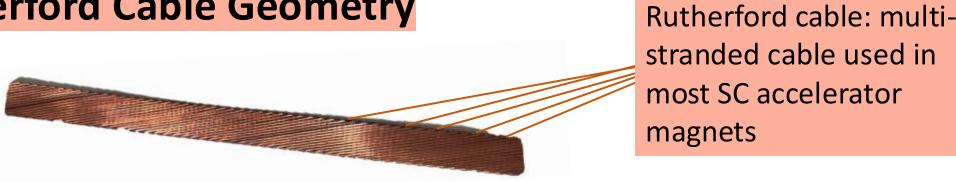
We will wind REBCO tapes around flat rounded-edge cable to minimize bent sections.
