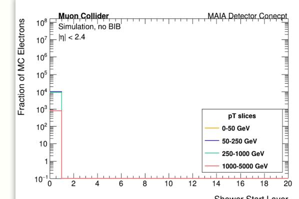
Electromagnetic showers start within the first 2 layers of the ECAL, proving the max profile start variable **is not** a source of error.
