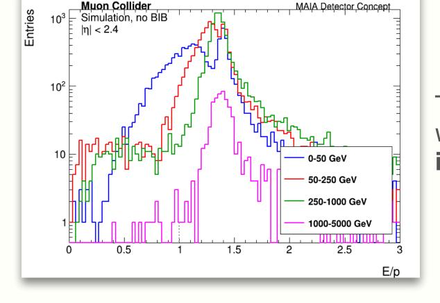
The E/p ratio is centered at ~1.4, which shows that the E/p variable **is** a source of error.
