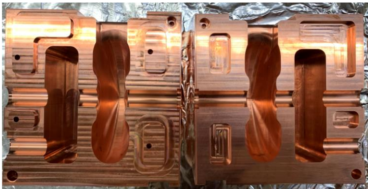
Split-block cavity halves prior to brazing
